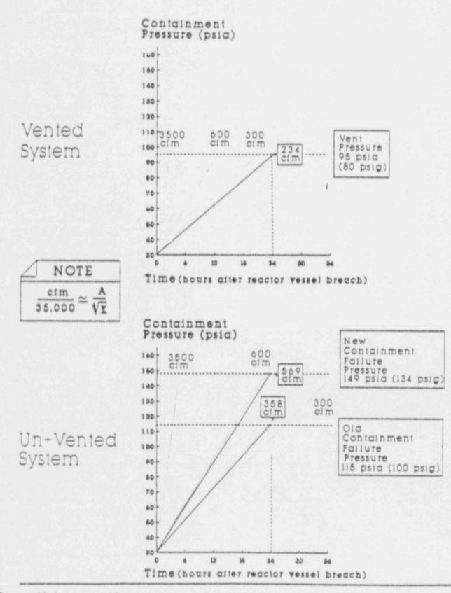
Figure 19.6-4 Wetwell pressure as a function of bypass flow (CFM) and time (hours).
