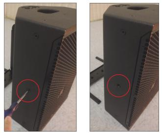
Pre-position the pieces pictured here onto each side of the –UB. Note that the knob for the thumb screw is pointed away from the speaker, while the rubber friction washer goes between the speaker and the metal surface of the –UB. The included metal washer goes between the thumb screw and the –UB.
