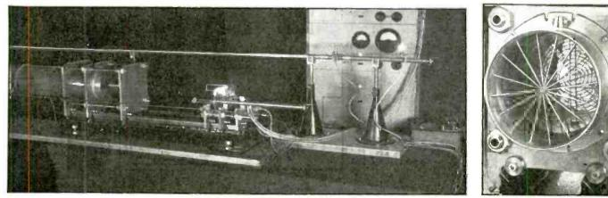
I.T.&T.'S NEW MICROWAVE GENERATOR In middle of photo above: 8-centimeter generator and its wavemeter; at left, coupling apparatus to a 12-cm. (dia.) dielectric guide; at right, receiving apparatus of a 16-mm. (inside dia.) dielectric guide. Extreme right: microwave transformer to convert Eo wave into Ho wave; and an Eo wave filter.
