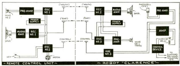
Block diagrams of the complete apparatus in (left) the innards of Clarence and (right) the innards of the radio remote control unit.
