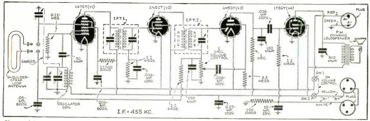
Diagram of the Motorola type 41-S model "Sporter" personal radio set. The chassis may be put into operation for servicing by plugging the loop back into place. Frequency range is 540 to 1,560 kc. Uses General batteries Nos. 2FI ("A"), 20AAA9, and 34AAA9 (latter 2 for "B").
