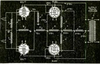
Fig. 1. Schematic diagram of the fundamental circuit of the direct-coupled 30-W, amplifier,
