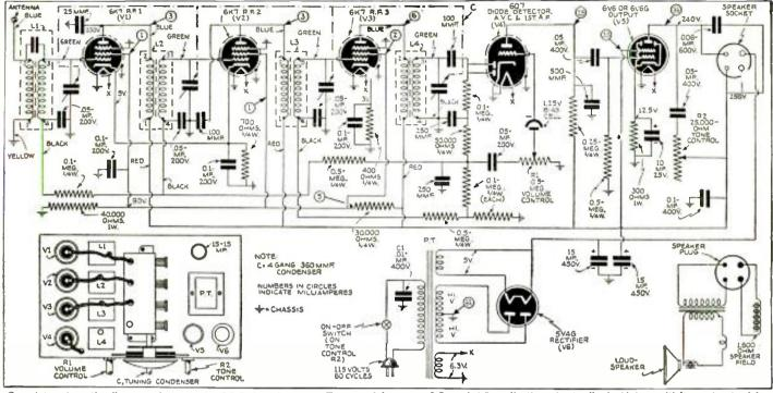
Complete schematic diagram of the 6-tube T.R.F. broadcast set. The use of iron-core R.F. and I.F. coils throughout affords high sensitivity and selectivity.
