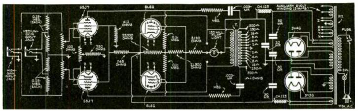
Fig. 2. Complete schematic diagram of the 30-W. all-push-pult direct-coupled amplifier.
