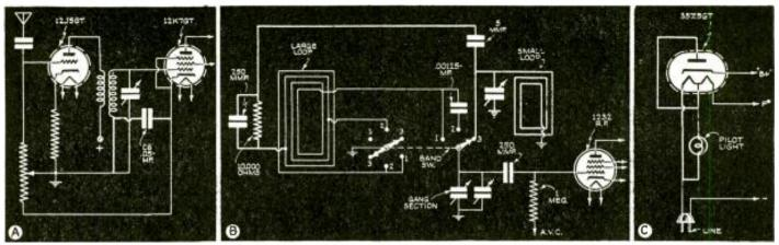
Fig. 1. New circuit features of (A) Emerson Model CU-265; (B) Philco Models 40-180, 40-185, 40-190; (C) General Electric Model H-400.
