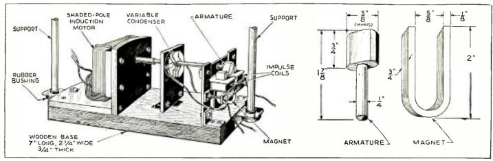
Fig. 1. Complete constructional drawing for building the frequency modulator (wobbler) and impulse generator.
