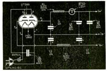
Diagram of Power Supply for operating battery-portables on A.C.-D.C. light
