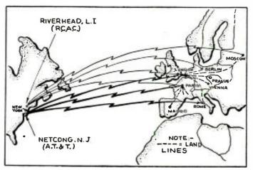
Radio circuits are shown solid; land tines are dotted. The A.T.&T. station at Netcong, N. J., has radio circuits to London and Paris only. The remainder of Europe is contacted by land lines. The R.C.A.C. station in Riverhead, L. I., has radio circuits to all the capitals of Europe.
