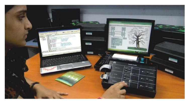
Elevator control module MC06 enables the students and practicing engineers to gain invaluable practical experience of the principles and application of Elevator and Microcontroller.
