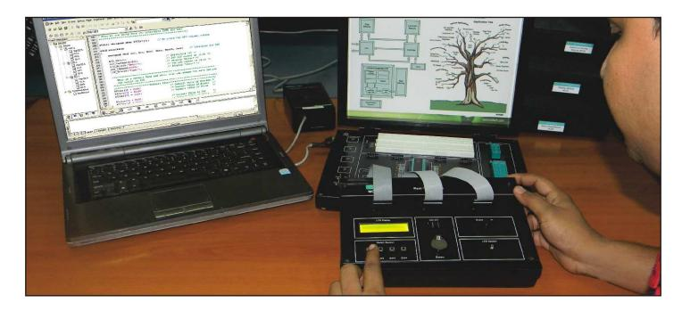
Real Time Clock module MC08 is an extension module for Nvis Microcontroller development platforms. It helps the user to gain invaluable practical experience of the principles and application of real time clock, LCD, switch and buzzer module in microcontroller based projects.
