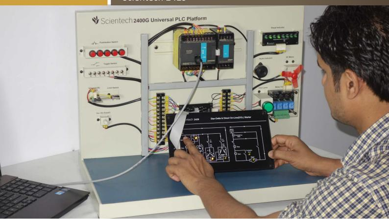
**Scientech 2429** Star Delta & Direct on Line (DOL) Starter enables Students and practicing Engineers to gain invaluable practical experience on application of Programmable Logic Controllers. The objective is to connect and program an external Programmable Logic Controller to monitor and control Motor Starter.
