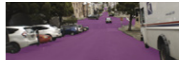
Can focus solely on the road surface even in complex road environments (Color-codes the recognized road surface on a pixel-by-pixel basis)
