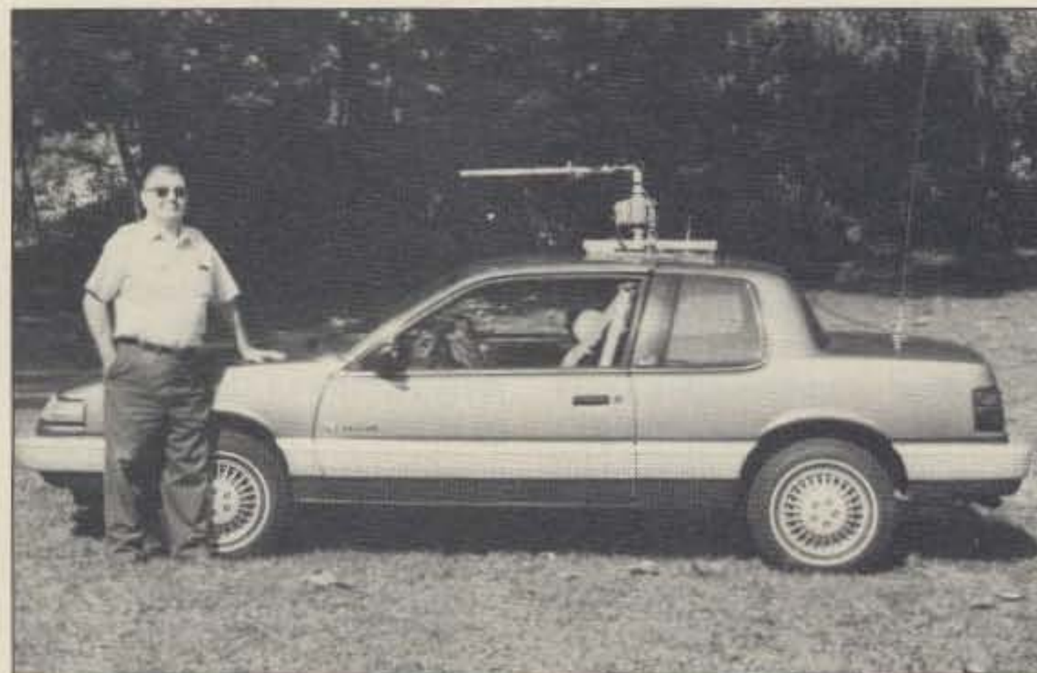
Photo A. Frank Williams WB9KCC and his detachable car-top beam and U-100 ROTOR. Note the use of bungie cords for quick installation.
