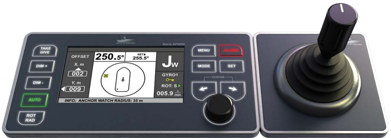
JP4000 main control panel
