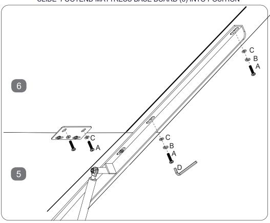
LOOSELY CONNECT (6) TO THE PLATES THEN SCREW OTHER x4 SETS OF BOLTS INTO PLACE
