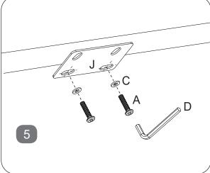
BEFORE FITTING FOOTEND BASE BOARD (6) FIT BOTH PLATES (J) TO HEADEND BASE BOARD (5) AS SHOWN
