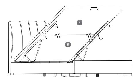
WHEN ALL x16 BOLT SETS ARE IN PLACE, MAKE SURE SIDES OF BASE BOARDS ARE IN LINE WITH EACH OTHER, THEN TIGHTEN ALL BOLTS 100%
