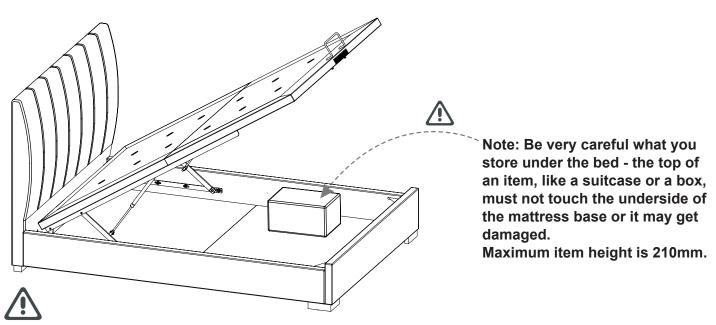
**NOTE**: Before fitting the mattress on top of the mattress base, carefully lower the base holding the handle firmly and if necessary hold base horizontal, then place mattress on top. Be careful, without a mattress in place the base may lift on its own and speed of movement is quick and may cause injury.
