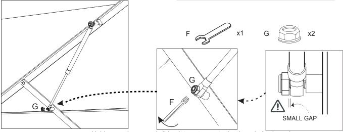
Hold up each arm and slide piston stem onto the threaded axle and fit loc-nut (G) using spanner (F).
