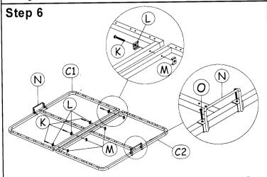
Assemble front & back frames bed base with bolts 'K' and fix base handles to the bed base with bolts 'O' as shown.
