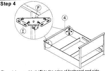
Fix metal corner block 'F' to the edge of footboard and side rails with bolts 'I' as shown.
