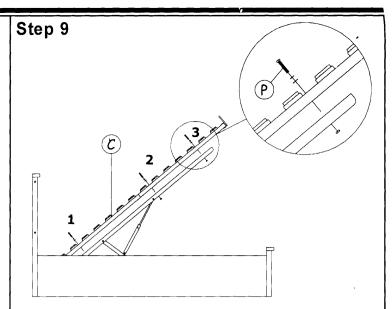
Assemble the bed base on the right & left hydraulic frame and fix bolts starting from  $\bf '1'$  to  $\bf '3'$  as shown. Important note : Do not tighten the bolts yet!
