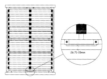
Adjust the bed base, make sure distance with the front footboard approximately 10 -15mm gap as shown. Important note: Tighten all screws.
