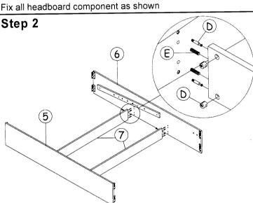
Assemble the left & right side rails to the center wood panel with minifix screws as shown.
