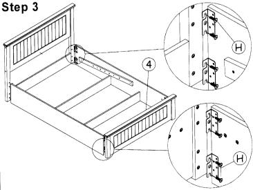
Fix side rails to the headboard and footboard with bolts 'H' as shown.
