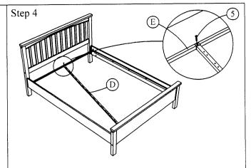
Fix center bar 'D' to cross bar 'E' by follow like diagram as shown.
