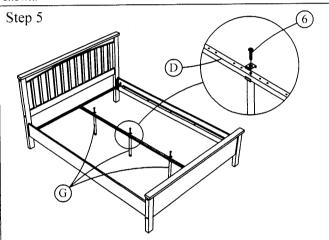
Fix in support leg with bolt 'G' as shown.
