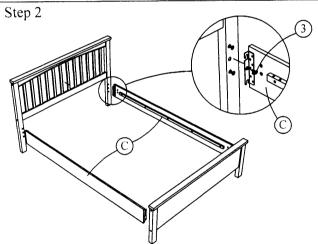
Hook the side rail to bolt as shown and don't tighten the bolt yet.
