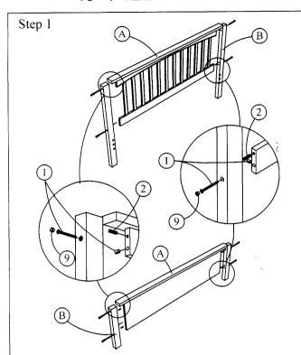
Assemble the bed frame headboard and footboard component as shown and tighten all bolt.
