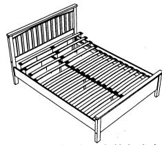
Once both wood slats have been inserted with the plastic caps, fix it on the wood side rails and center bar by pressing it accordingly to the default holes. Ensure the plastic cap's pin is aimed to the hole. At last make sure all screws and bolts are tighten.
