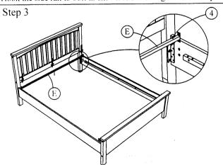
Put in cross bars and fix in bolt '4' as shown in diagram and tighten all bolts.
