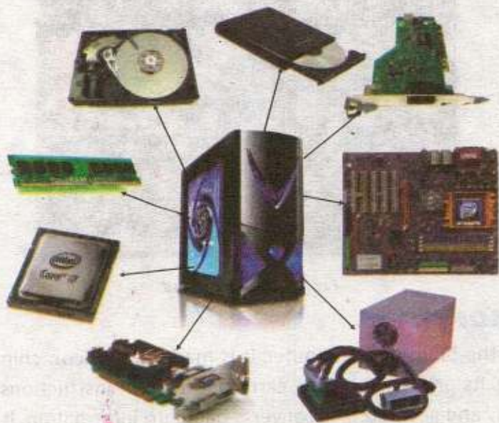
Fig. 1.2.3a System Unit and its Components
