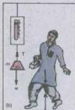
acceleration downward w - T = ma T = w - ma
