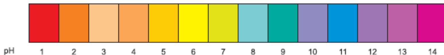
Fig. 10.3. Colours of universal indicator
