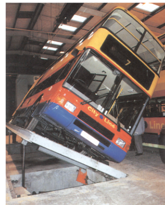
Figure 4.35: A double decker bus being under test for stability.
