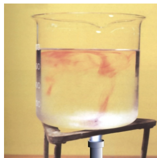
Figure 9.7: Crystals of potassium permanganate are used to show the movement of water on heating.
