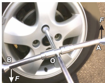
Figure 4.25: A double arm spanner.
