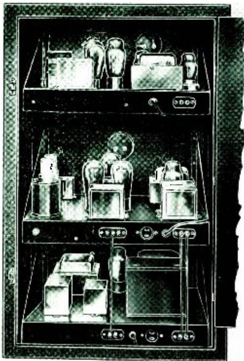
Figure 1 Rear view of the transmitter with the carrier-control unit but without the 200 watt amplifier.
