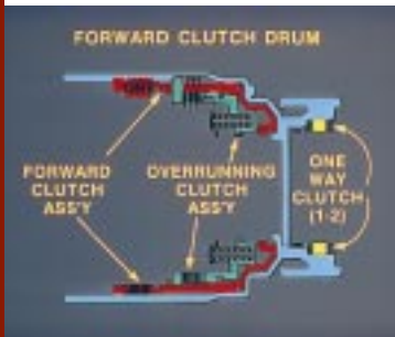
Forward Clutch Drum
