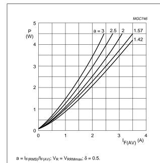
Maximum steady state power dissipation Fig.4 (forward plus leakage current losses, excluding switching losses) as a function of average forward current.
