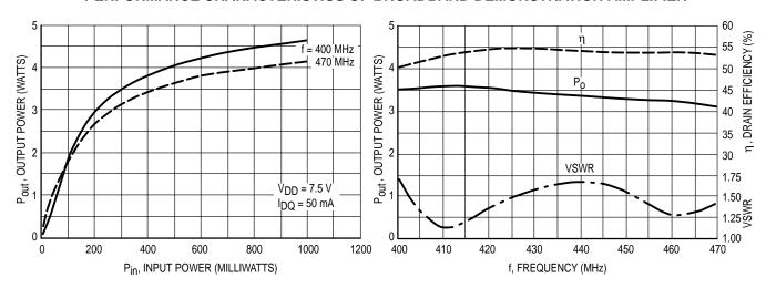
Figure 14. Output Power versus Input Power
