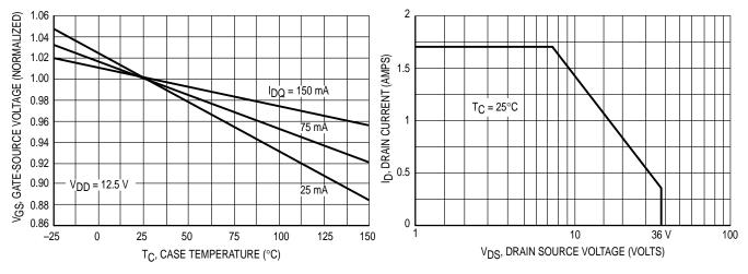
Figure 10. Gate-Source Voltage versus **Case Temperature**
