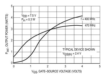
Figure 16. Output Power versus Gate Voltage
