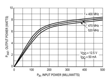
Figure 3. Output Power versus Input Power
