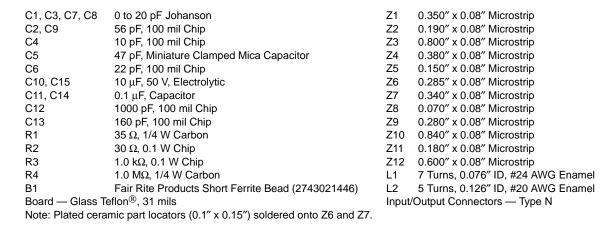
Figure 1. 512 MHz Narrowband Test Circuit
