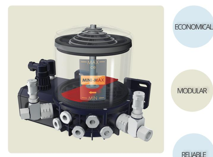
The **Mini-Max** electric pump was designed to work both as a multi-outlet system and with **DPX** progressive distributors. Naturally both systems can also be combined. It is driven by a 12 V DC or 24 V DC gearmotor and is capable of pumping grease with a max consistency of NLGI 2. On demand it can be supplied with a Timer.
