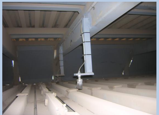
Stainless brushes apply oil on guide rails and chain
