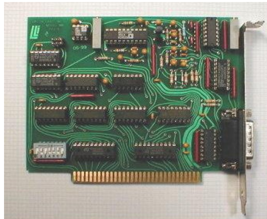
Model 141 20-bit Delta Sigma converter at 3.5 kHz with 4 input channels, 2 of the channels are dedicated for self-calibration.
