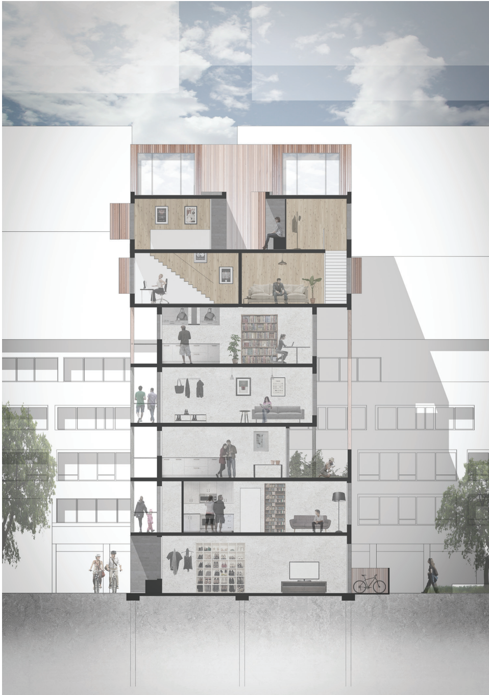
FIGURE 34. Using lightweight engineered timber construction allows the existing building to be extended without resorting to environmentally wasteful demolition.
