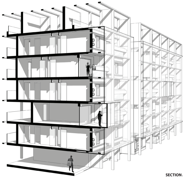
FIGURE 23. Cutaway section of the proposed Elmington Estate. The existing concrete frame is retained and residential units are extended with engineered timber pods.
