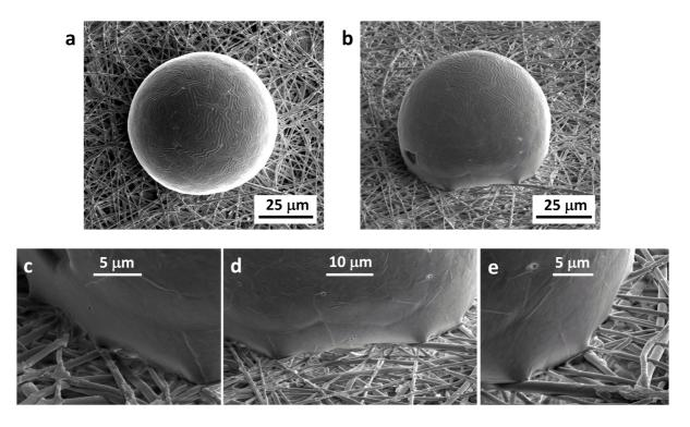
**Figure 4.** 2D cryo-SEM micrographs of sprayed silicone oil on plasma treated electrospun nylon 6 nanofibers **in a)** and **b)**. Higher magnification cryo-SEM imaging in **c)**, **d)** and **e)** indicates the contact line between silicone oil and nanofibers
