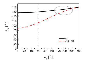
**Figure 7.** Plot of a liquid contact angle on a porous surface, described by the liquid fraction in contact with air  $f_2$ , equal to 0.96 (or fraction of nanofibers  $f_2 = 0.04$ ) and  $\theta_Y = \theta_{nano} = 60^{\circ}$  for silicone oil on nylon 6 nanofibers, indicated with a dotted line. The superoleophobic region where  $\theta_{CB} \ge 150^{\circ}$  is circled at the top right corner of the plot.
