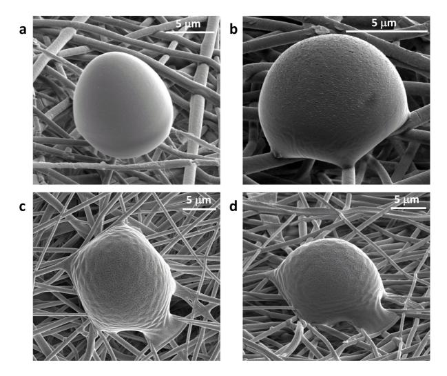
**Figure 5.** Scanning electron micrographs of silicone oil droplets contacting nanofibers network of plasma treated electrospun fibers. **a)** side view of a non-wetting droplet suspended on nanofibers, **b)** side view of an oil droplet with wetting contact points on individual nanofibers with **c)** top view and **d)** side view of a further oil droplet wetting nanofibers.
