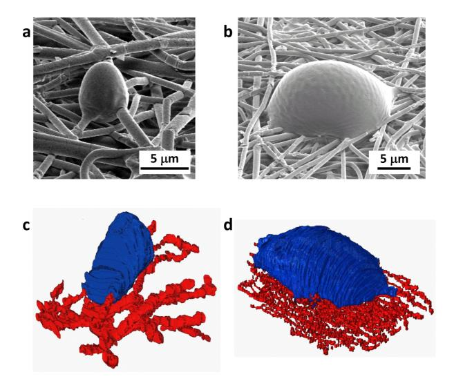
**Figure 3.** 2D cryo-SEM micrographs in **a**) and **b**) showing individual silicone oil droplets before slice and view imaging. 3D reconstructions of the individual droplets in **c**) and **d**) showing silicone oil droplets (in blue) on a plasma treated electrospun nanofiber array (shown in red).
