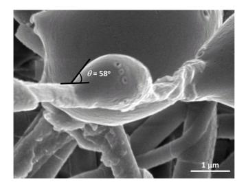
**Figure 6.** Scanning electron micrograph of a relatively small silicone oil droplet contacting an individual plasma treated electrospun nanofiber. Contact angles indicate partial wetting that was consistent with Wilhelmy balance measurements.
