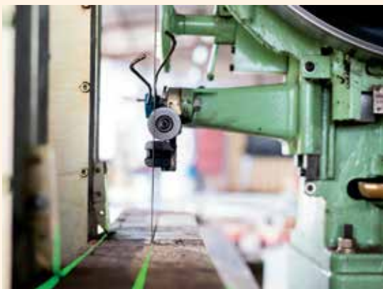
Laser guides help the sawyers make more accurate cuts
