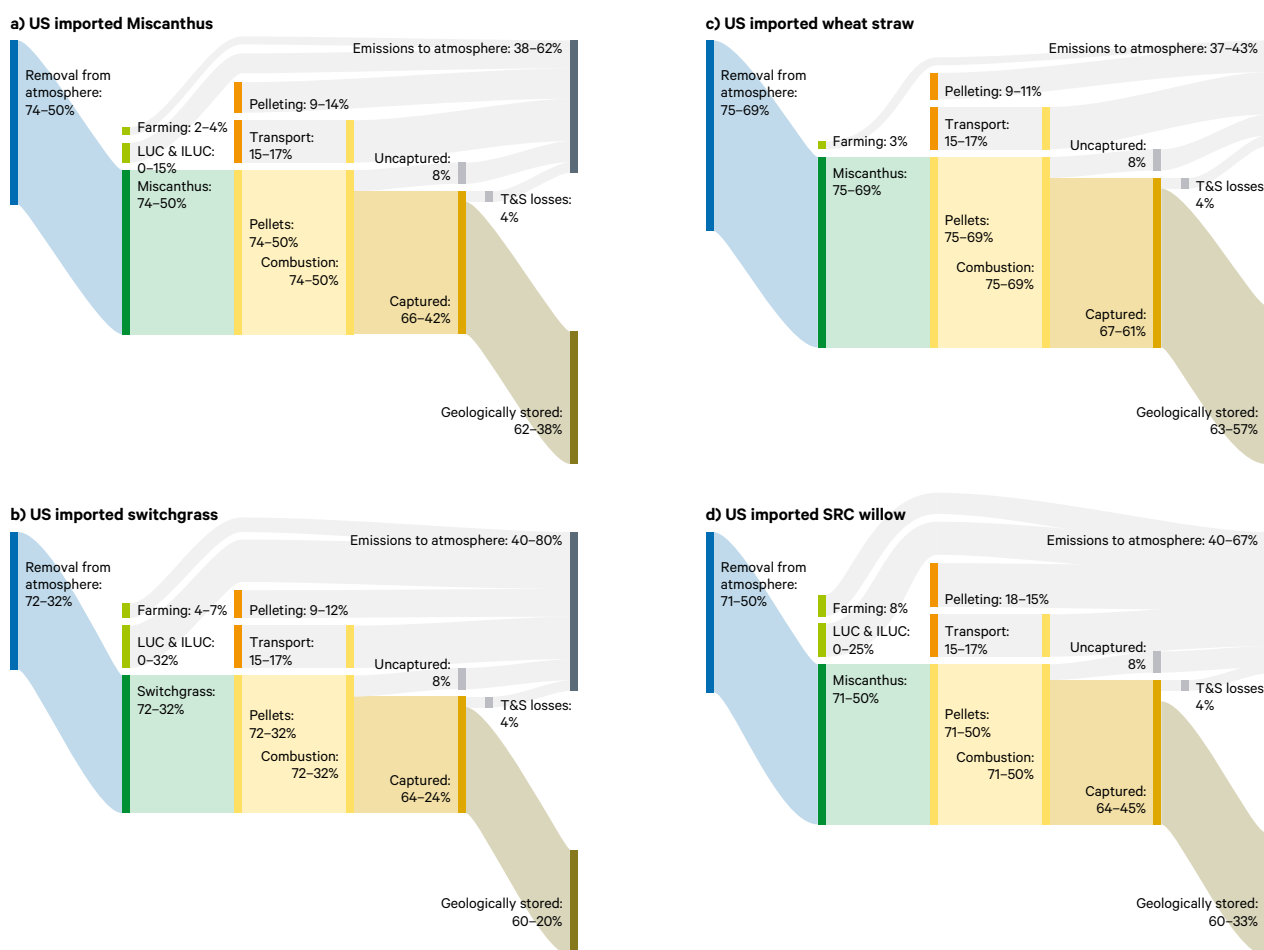
Figure A1. Carbon efficiency of UK BECCS based on (a) miscanthus, (b) switchgrass, (c) wheat straw and (d) short rotation crop (SRC) willow, grown in the US and imported to the UK
