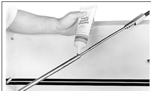
ABYC-approved mechanical steering cable.
