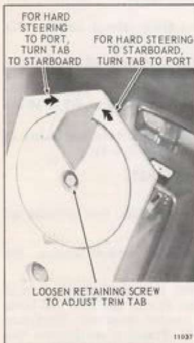
Figure 6-77. Trim Tab Adjustment
