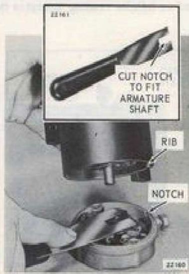
Figure 7-14C. Assembling Commutator End (Bosch)
