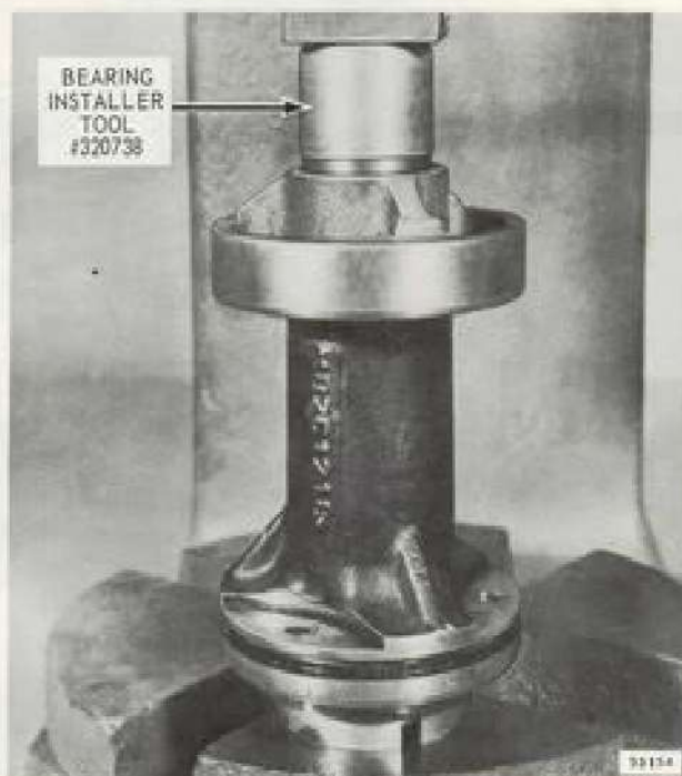
Figure 6-37. Installing Aft Bearing
