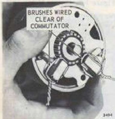
Figure 7-11. Reassembling Starter (Prestolite)
