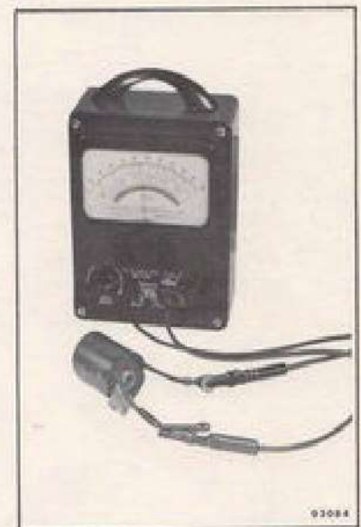
Figure 3-17. Testing Choke Solenoid
