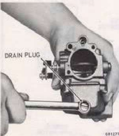
Figure 3-8. Drain Carburetor
