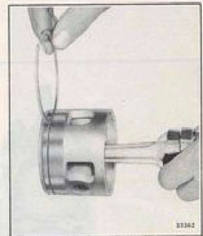
Figure 5-31. Checking Fit of Ring in Lower Groove
