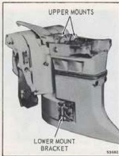
Figure 6-7. Upper and Lower Rubber Mounts (Short Shaft)
