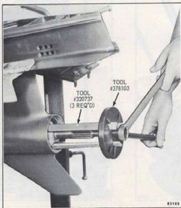
Figure 6-18. Removing Bearing Housing
