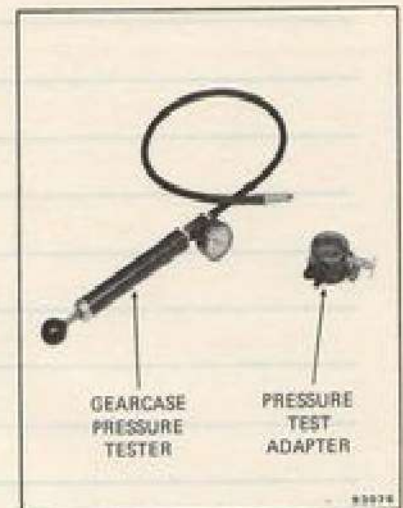
Figure 3-28. Pressure Test Equipment
