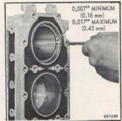
Figure 5-30. Checking Ring Gap in Cylinder
