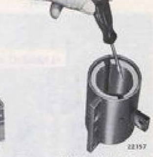
Figure 7-9B. Checking Permanent Magnets
