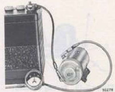
Figure 7-5. Starter Motor Test
