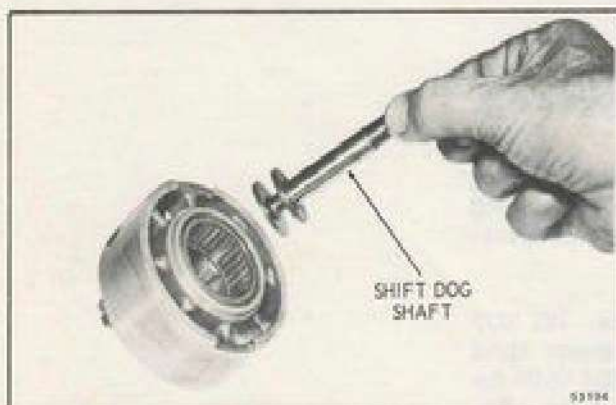
Figure 6-64. Installing Shift Dog Shaft
