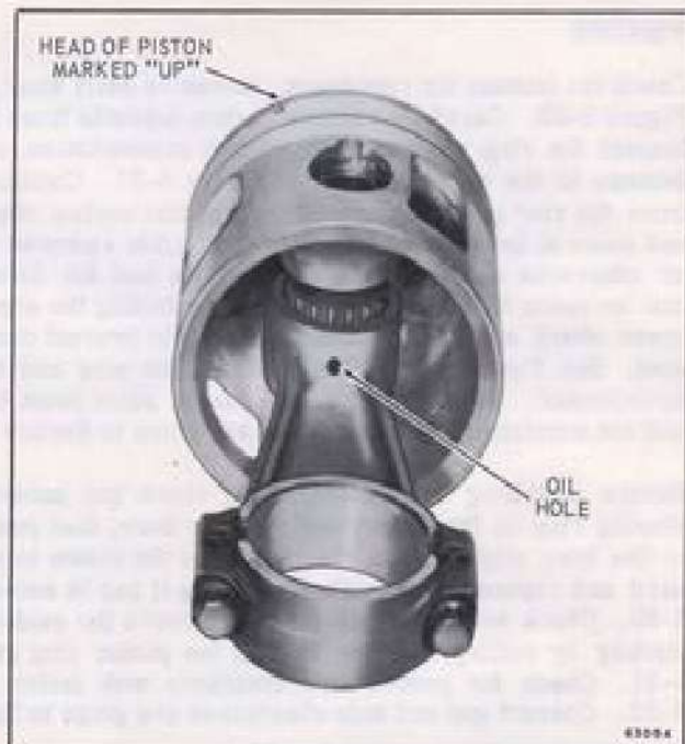
Figure 5-34. Oil Hole in Connecting Rod
