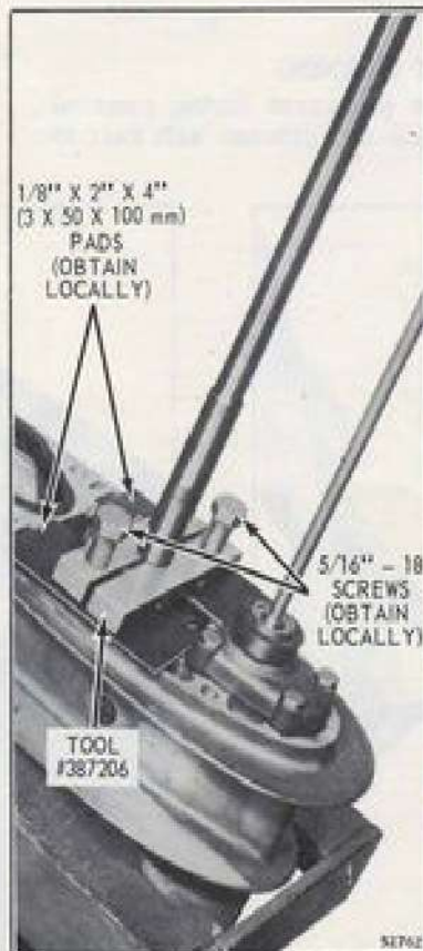
Figure 6-22. Driveshaft Puller
