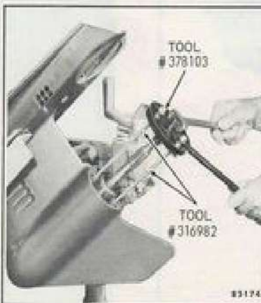
Figure 6-54. Removing Propeller Shaft Bearing Housing
