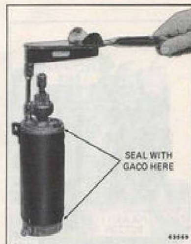
Figure 7-15. Torquing Thru-Bolts (Bosch)
