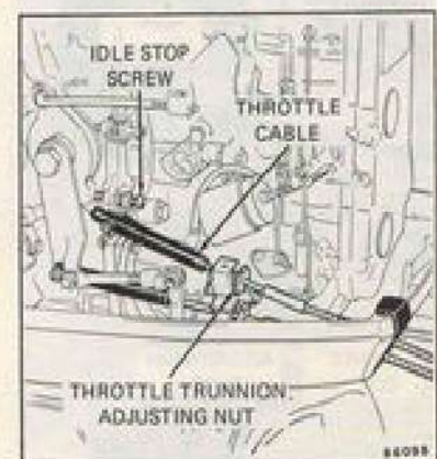
Figure 2-11. Throttle Cable Adjustment
