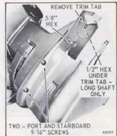
Figure 6-5. Gearcase Screws
