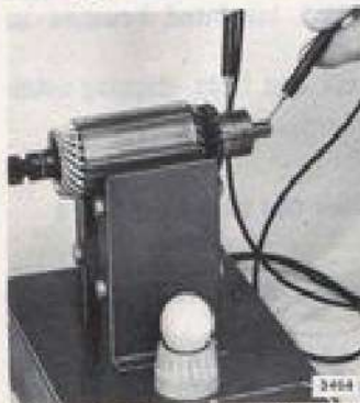
Figure 7-8A. Checking for Grounding
