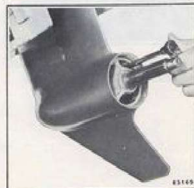
Figure 6-17. Removing Bearing Head Screws
