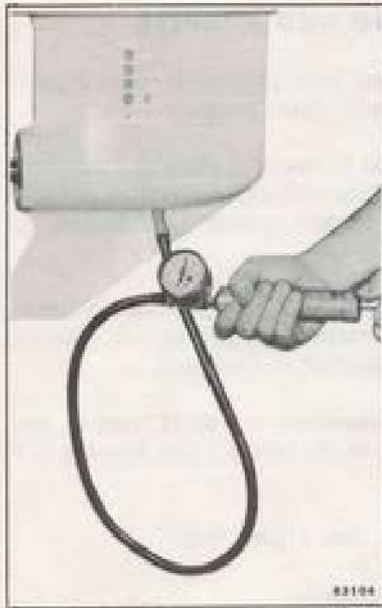
Figure 6-74. Pressure Testing Gearcase
