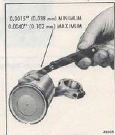
Figure 5-32. Checking Groove Side Clearance
