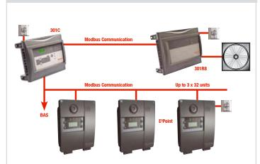
Supports Modbus protocol to daisy-chain E³Point detectors, providing up to 96 points of monitoring on a serial bus. Excellent option for controller-based (VA301C) installations common in larger applications. A relay output is provided as an option for activating ventilation directly (e.g. when fan is located in close proximity to detector).
