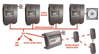
$E^3$ Point outputs directly to BACnet or other BAS. Alarms, strobes and horns are activated through BAS with link to DCV/HVAC controls. This system design supports new and retrofit installations for large buildings, and can couple with a controller to effectively integrate wired and wireless system components. A relay output is provided as an option for activating ventilation directly (e.g. when fan is located in close proximity to detector).
