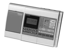
The Xtralis VESDA VLP detector is the central element of the Xtralis VESDA ASD product range. Using unique detection principles, the VLP has an alarm sensitivity range of 0.0015%–6.25% obscuration/ft (0.005%–20% obscuration/m). The VLP is classed as a "Very Early Warning Smoke Detector". This means that it detects fire at the earliest possible stage and reliably measures very low to extremely high concentrations of smoke.
