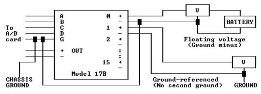
FIGURE 2. TYPICAL INPUT CONNECTIONS
