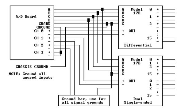
Read differential inputs 0-15 at A/D channel 0 Read single-ended inputs 0-15 of + bank at A/D channel 1 Read single-ended inputs 0-15 of - bank at A/D channel 2
