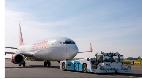
The Taxibot has four-wheel steering, which makes it highly flexible. It can both turn on its axis and drive sideways. The Taxibot connects to the aircraft in such a way that the pilot can steer it with the nose wheel, and the Taxibot's flexibility ensures that it follows the movements of the nose wheel exactly.
